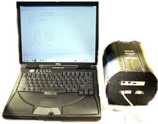
Figure 2 SwRI™ Rapid Prototyping Electronic Control System (RPECS™) is used to control the 42 V AC System
